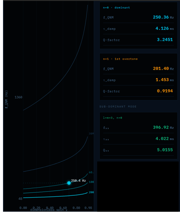
Figure 5. Kerr parameter and mode table for the simulated black hole. The highlighted point shows the dominant quasi-normal mode frequency for M_f=68.5M_\odot and \chi=0.69 , giving f_{\text{QNM}}=250.36 Hz and damping time \tau=4.126 ms. The table also compares the dominant mode, first overtone, and l=m=3 subdominant mode, showing that different quasi-normal modes have different frequencies, damping times, and quality factors.
