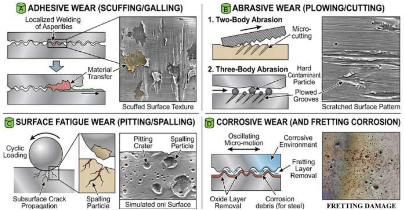
Fig.8. Wear Mechanisms and Surface Degradation Patterns
